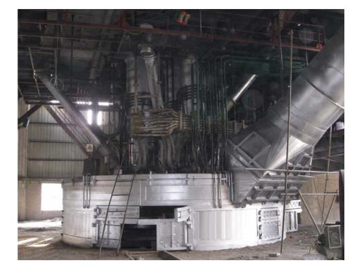
Ferroalloy Submerged Arc Furnace
