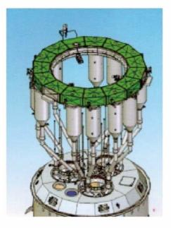
Schematic Diagram of Electrode Column
