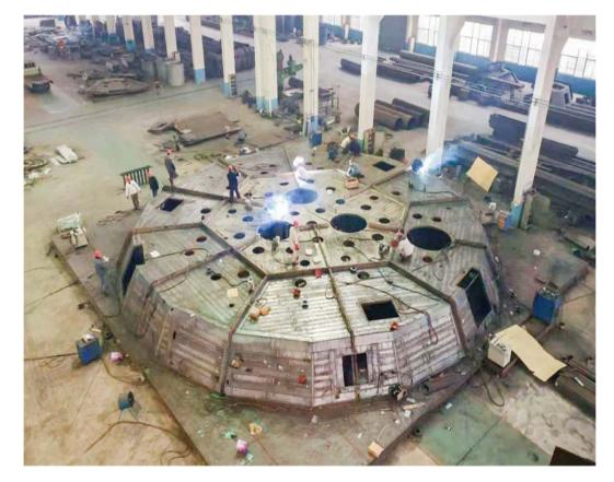
Manufacture and Assembly of Large Airtight Submerged Arc Furnace Cover Factory
