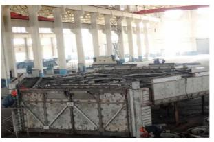
Large all stainless steel semi-closed furnace cover factory production and assembly
